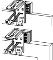
combination of the bracket and spacer block with two 2" screw.
