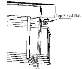
Gently insert the flat screwdriver into the back slot of the installation bracket and turn clockwise. Remove the shade as below drawing.
